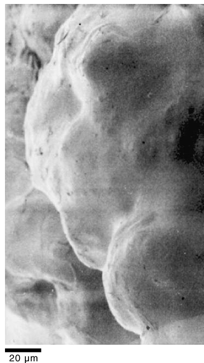
Figure 3. Scanning electron micrograph of theophylline microcapsules in the particle size range of 500–800 \mu\text{m} .
